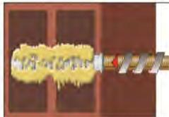
7. The position of the embedment depth shall be marked on the threaded rod. Push the threaded rod into the anchor hole while turning slightly to ensure positive distribution of the adhesive until the embedment depth is reached. The anchor shall be free of dirt, grease, oil or other foreign material.
