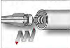
1. Remove the cap and attach the supplied static-mixing nozzle to the cartridge and load the cartridge into the correct dispensing tool. In case of a foil tube cartridge, cut off the clip before use. For every working interruption longer than the recommended working time (Table B4 and B5) as well as for new cartridges, a new static-mixer shall be used.
