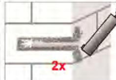
4. Blow out from the bottom of the bore hole two times. Attach the appropriate sized brush ( $> d_{b,min}$  Table B2 or B3) to a drilling machine or a battery screwdriver, brush the hole clean two times, and finally blow out the hole again two times.
