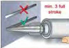
2. Initial adhesive is not suitable for fixing the anchor. Prior to dispensing into the anchor hole, squeeze out separately a minimum of three full strokes, for foil tube cartridges six full strokes and discard non-uniformly mixed adhesive components until the mortar shows a consistent grey colour.
